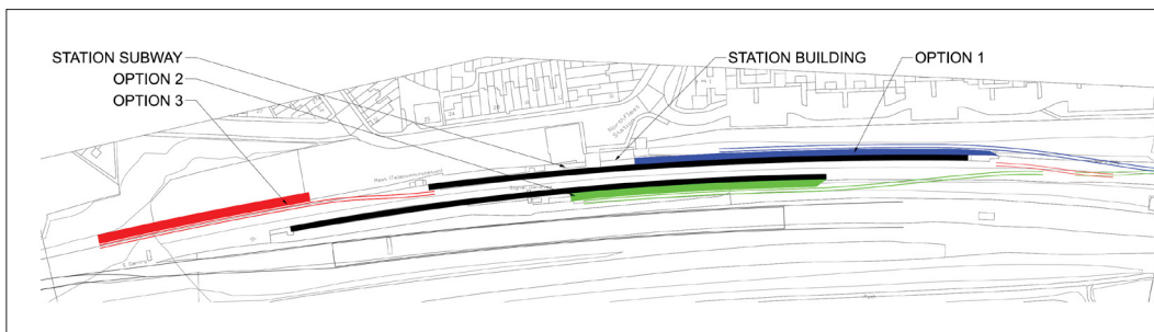
Figure 15 - Dedicated Platform Options at Northfleet Station - An image showing a map with the existing and proposed platform options. To the left in red is option 1, in the lower middle in green is option 2, in the upper middle in blue is option 1.
