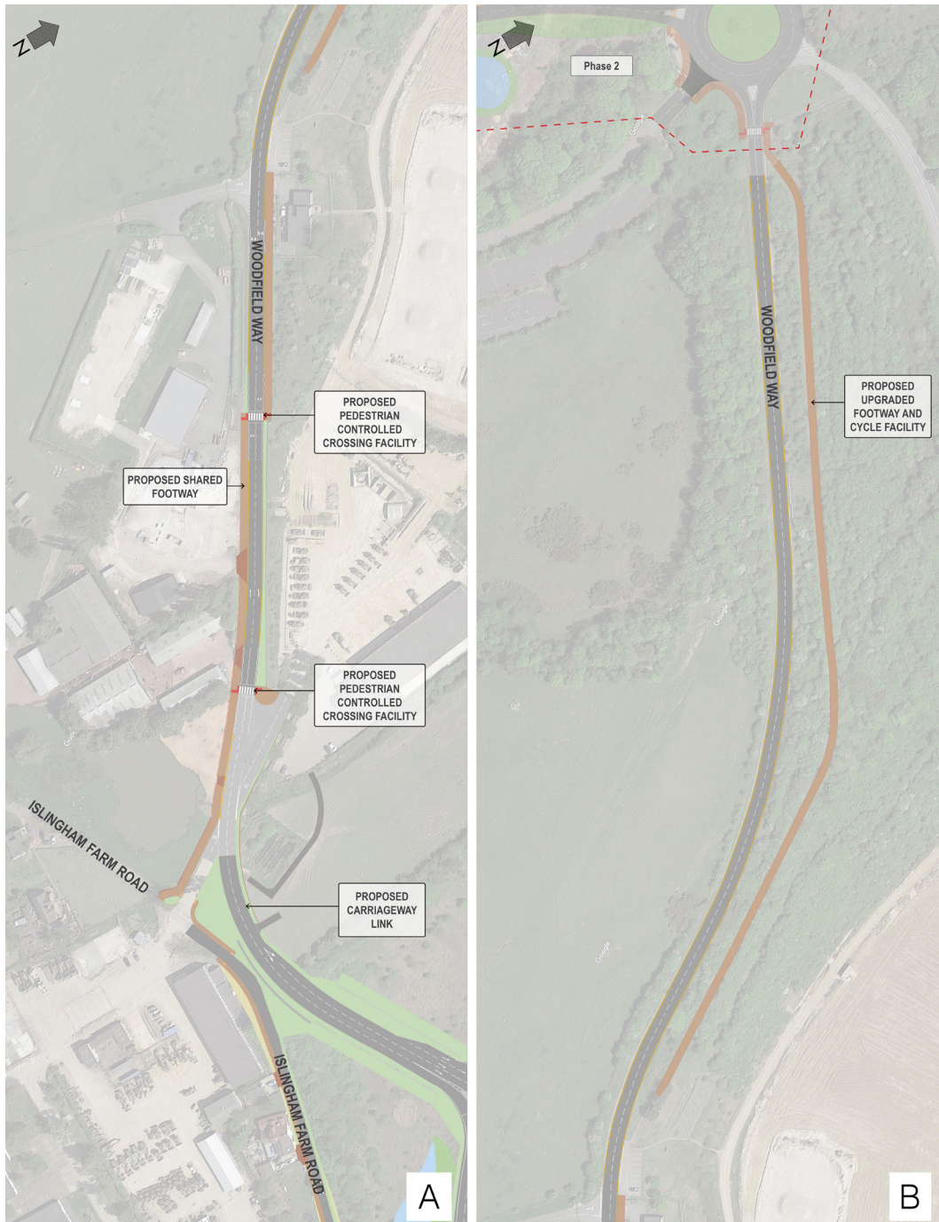
Figure 17 - view A and B shows local improvements on Islingham Farm Road and shows the improvements along the existing Woodfield Way including the provision of several crossing points. In addition, the introduction of an adjacent shared footway cycleway facility will provide links with Islingham Farm Road and facilities further north to improve cycling connections through the area.
