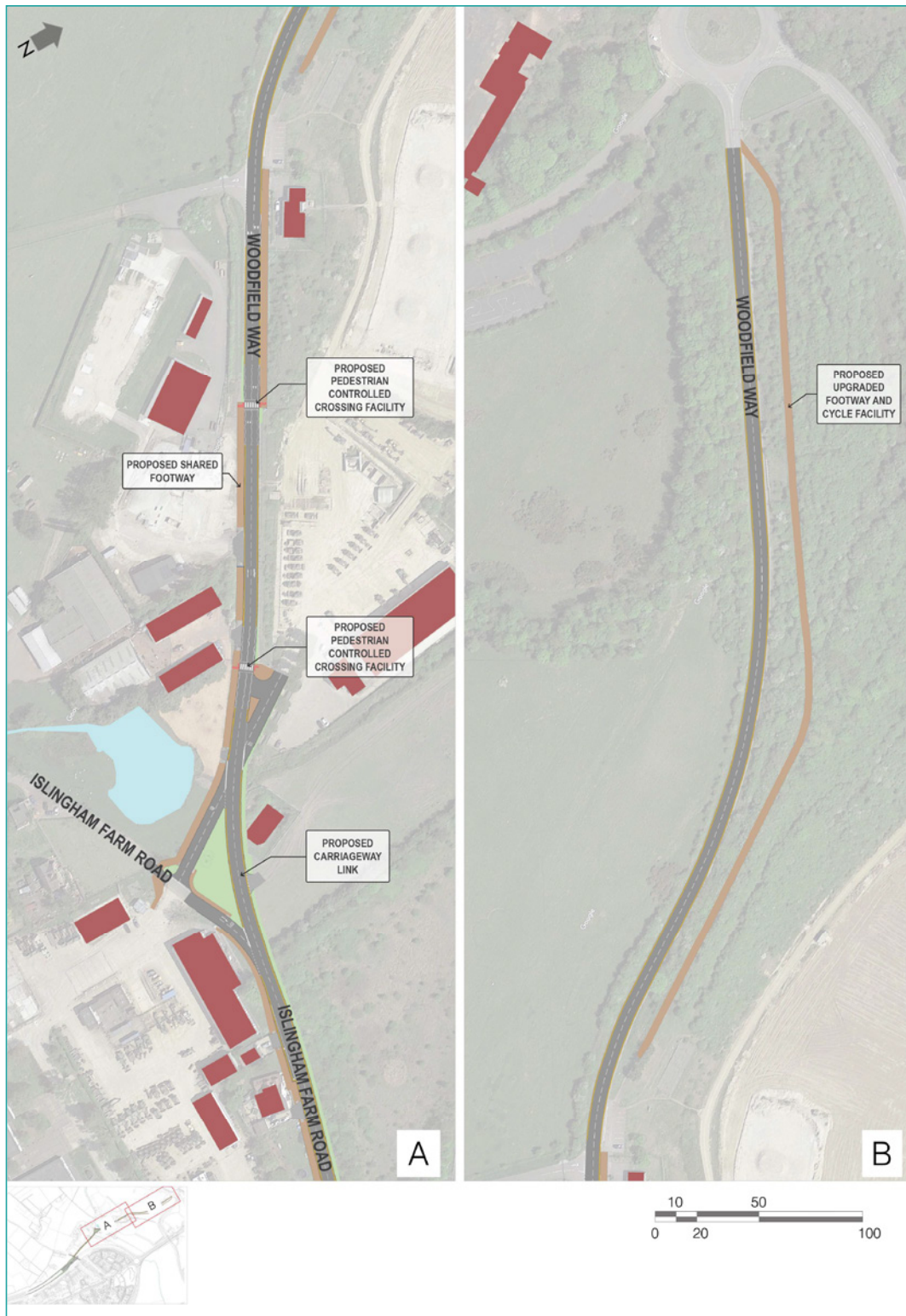
Figure 4: Phase 2 - View A shows the widening of Islingham Farm Road, realigned with Woodfield Way to provide improved traffic flow.
